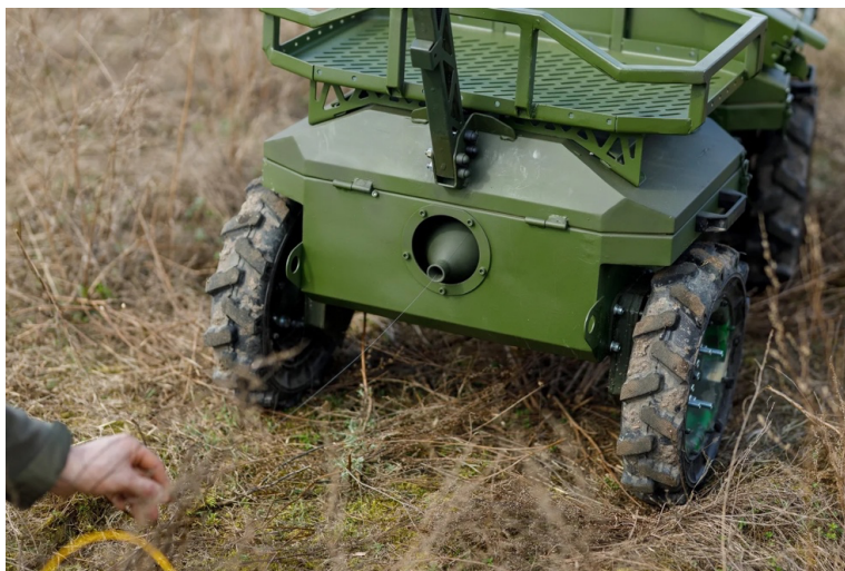
Figure 1. Use of fiber-optic technology in ground-based and aerial military drones. Source: https://focus.ua/digital/700214-optovo-lokonnye-drony-v-ukraine-ispytali-no-vye-bpla-foto
